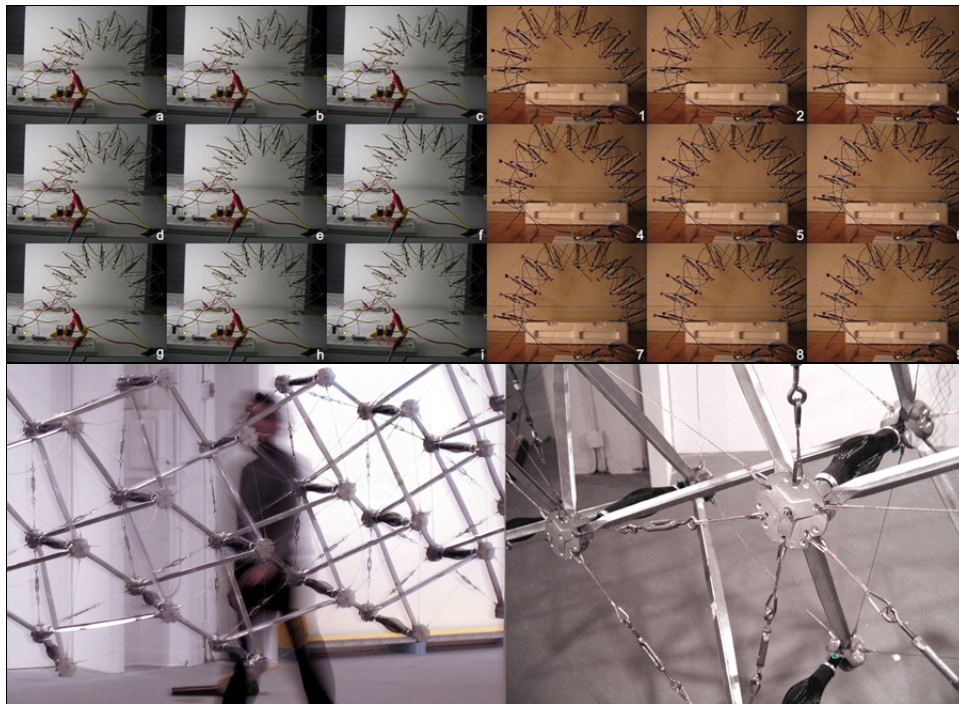
Figures 2a & 2b) Depicting class 3 systems as actuated systems changing shape via expansion and leaning. Figure 2b Depicts a full-scale actuated class 3 structure built by this author using cast aluminium components, pneumatic air muscles, stainless steel cable and hardware (2004).
